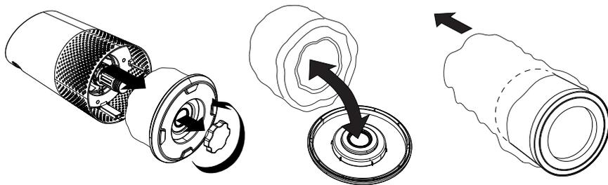
Unscrew bottom cover and remove plastic bag from filter.
